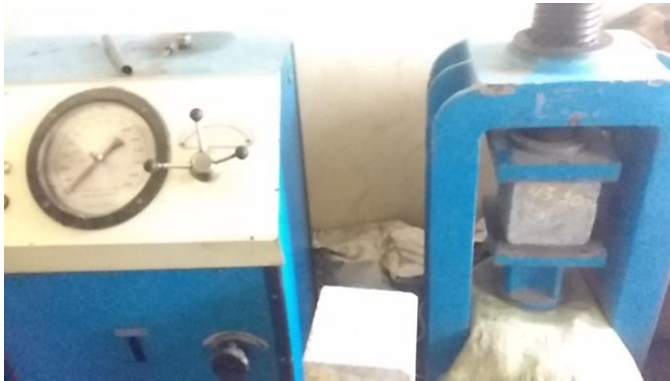
Figure 2 Compressive testing setup using universal testing machine
